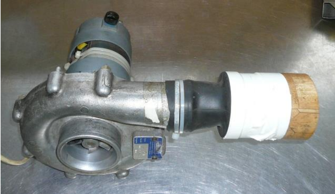
Motor driven blower unit used for starting
